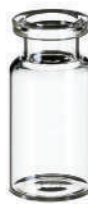
10 ml Headspace Vial, 46 x 22.5 mm clear glass, 1 st hydrol. class, DIN crimp neck, rounded bottom
