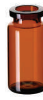
10 ml Headspace Vial, 46 x 22.5 mm amber glass, 1 st hydrol. class, DIN crimp neck, long neck, flat bottom
