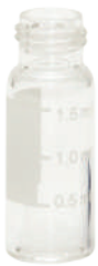
1.5 ml, Short Thread Vial ND9, 32 x 11.6 mm, clear glass, 1 st hydrol. class, wide opening, label + filling lines
