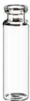
20ml Headspace-Vial, 75.5 x 22.5mm, clear glass, 1st hydrol. class, DIN-crimp neck, long neck, flat bottom
