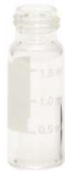
1.5 ml, Short Thread Vial ND9, 32 x 11.6 mm, clear glass, 1st hydrol. class, wide opening, label + filling lines
